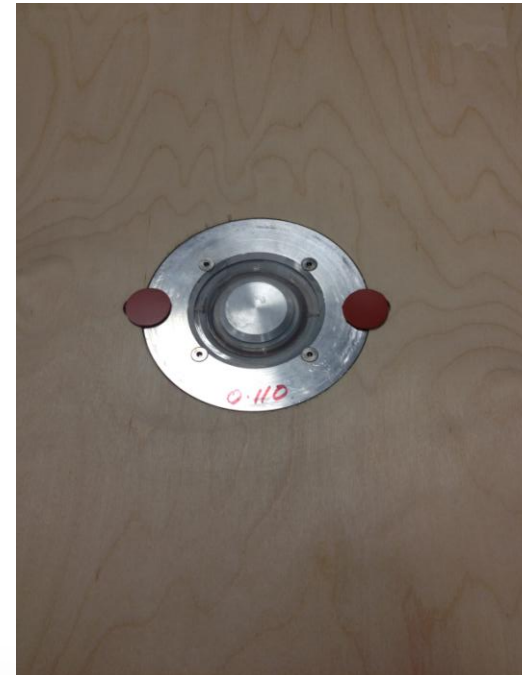
MF Open Diaphragm. 2Pi anechoic chamber measurement
