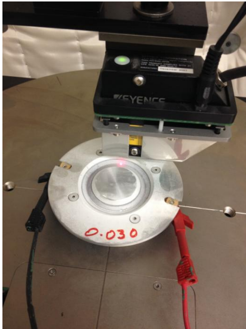
HF Open Diaphragm scanning by Klippel scanner
